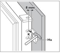
13. Place the small square on the guide again and fix it with the screws supplied.
